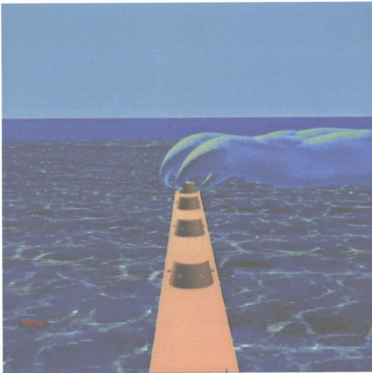
Figure 4.4: A snapshot from the system. This shows the jets are confined within a certain layer in the water, which is the result of different input parameters.
